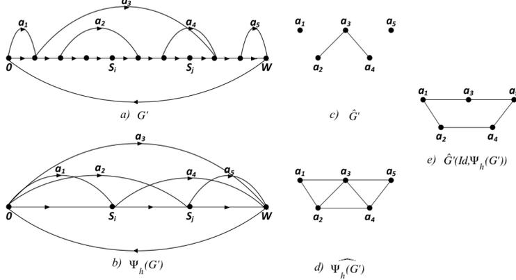
Figure 2: Heuristic aggregation. Subfigure a) is the original multigraph  $G$ , with its conflict graph c). Subfigure b) is the aggregated multigraph obtained using  $\mathcal{S} = \{0, \mathcal{S}_i, \mathcal{S}_j, W\}$ , with the corresponding conflict graph d). The conflict difference graph is e).
