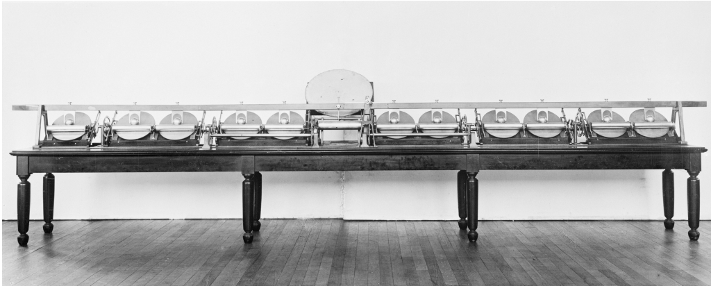
Fig. 0.7 William Thomson's first Harmonic Analyzer. 1876
